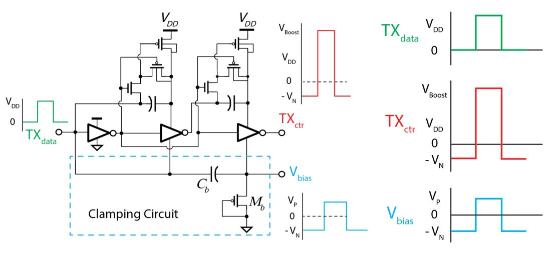
→ Helps reduce <u>off-leakage</u> up-to 92% during TX inactive phase
