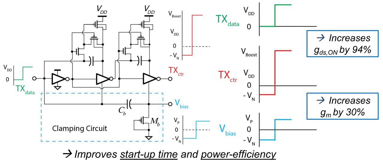
• When  $TX_{data} = 0$ , the  $V_{bias}$  is set to  $\sim -V_{th}$
