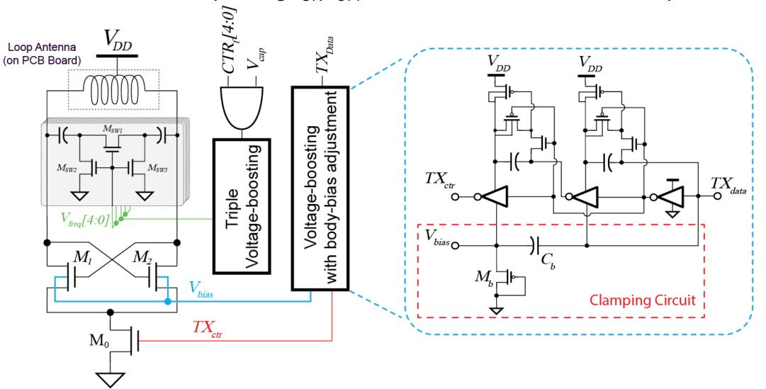
• When  $TX_{data} = 1$ ,  $TX_{ctr}$  is boosted 3× and  $V_{bias}$  is set to  $\sim V_{th}$
