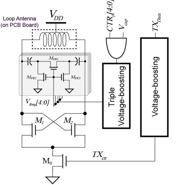
• TX control circuit for improving  $I_{ON}/I_{OFF}$  ratio of transistors and start-up time
