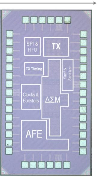
TSMC 65nm LP CMOS 1 mm<sup>2</sup> with pads
