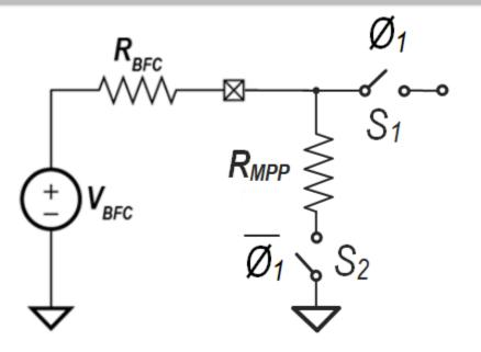
• Matched load  $R_{MPP}$  at only 1% duty ratio in this work
