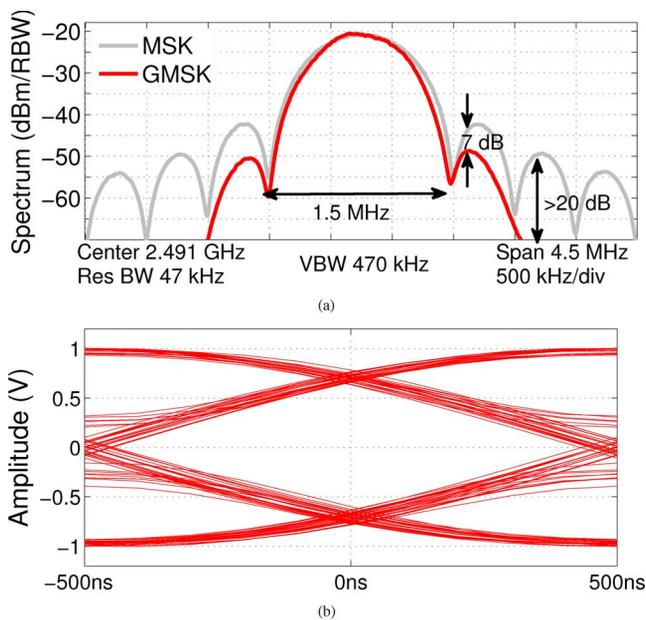
Fig. 19. 1 Mb/s GMSK. (a) Spectrum compared to MSK. (b) Eye diagram.
