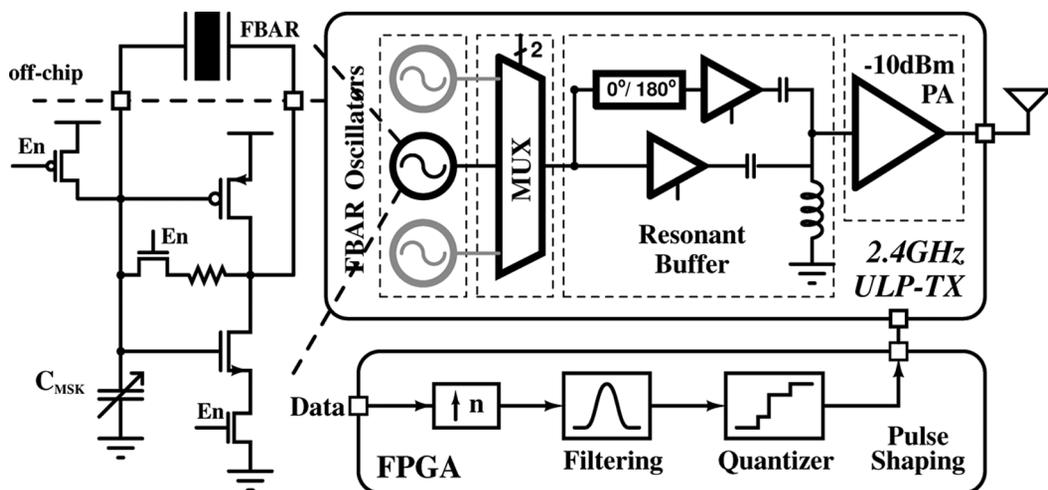
Fig. 3. TX architecture with the FBAR oscillator of one channel.
