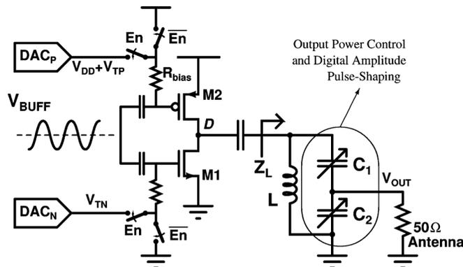
Fig. 11. Integrated PA with pulse-shaping using dynamic impedance transformation.
