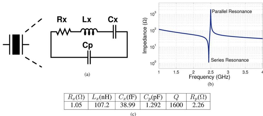
Fig. 2. Circuit model for RF resonators and the impedance profile of a representative FBAR. (a) Butterworth Van Dyke model for resonators. (b) Impedance characteristics of a representative FBAR. (c) Sample model values for FBARs used in this work.
