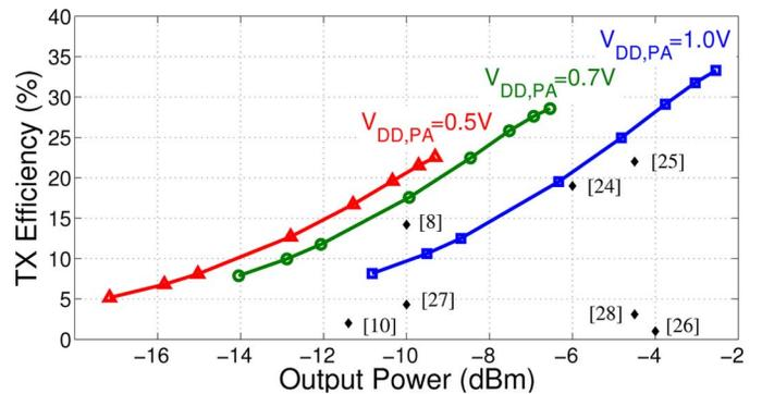
Fig. 15. Overall efficiency of the transmitter plotted for various  $V_{DD,PA}$  and impedance transformation settings. Results are also compared to previous frequency-stable TXs.
