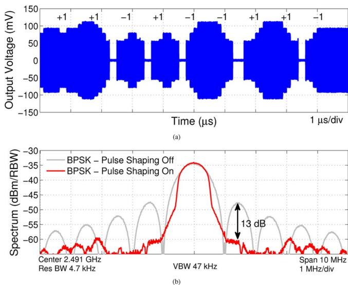
Fig. 18. 1 Mb/s BPSK with SRRC filtering. (a) 1 Mb/s BPSK modulated waveform with SRRC filtering. (b) 1 Mb/s BPSK spectra with and without pulse-shaping.
