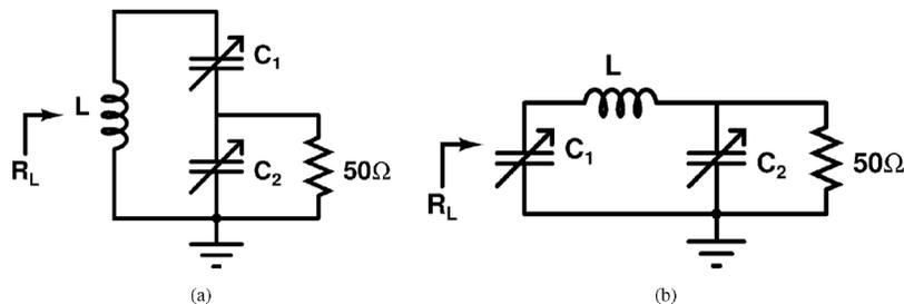
Fig. 8. Tapped capacitor and  $\pi$  matching networks. (a) Tapped capacitor match. (b)  $\pi$ -match.
