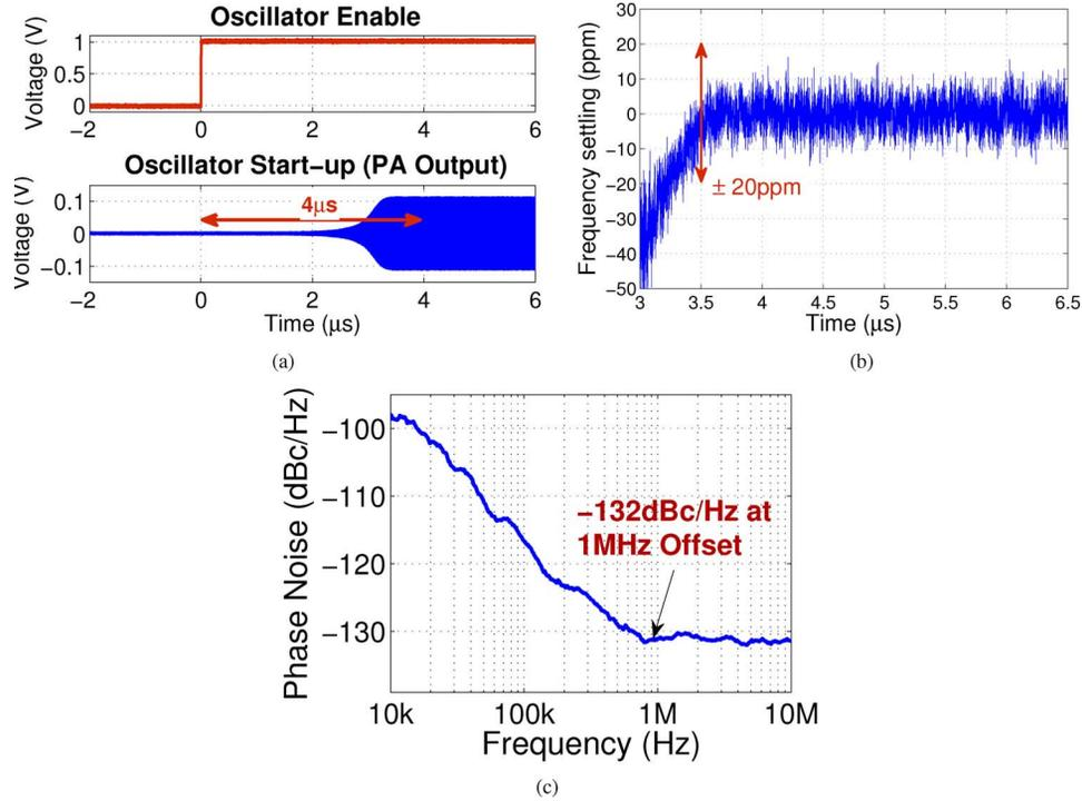
Fig. 13. Measurement results of FBAR oscillator. (a) Startup time. (b) Frequency settling transient. (c) Phase noise measured at the output of the transmitter.
