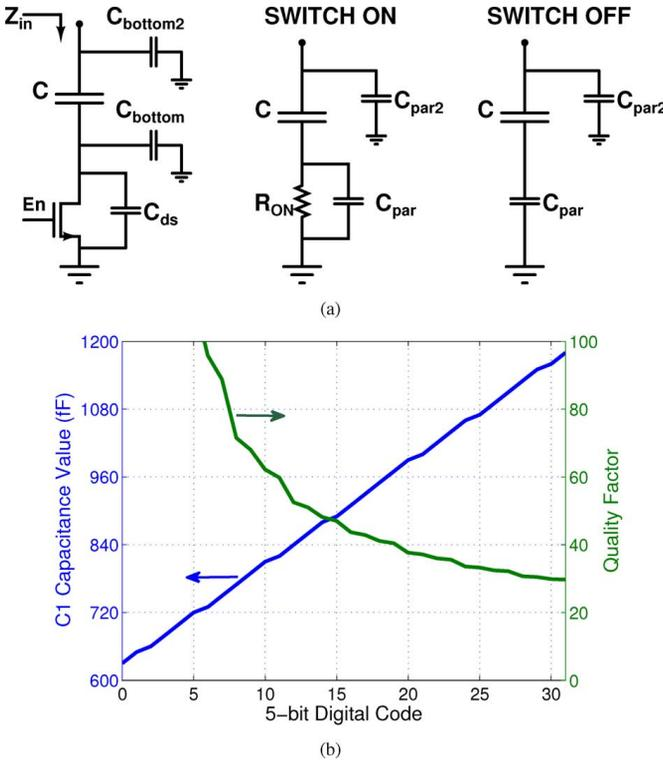
Fig. 10. (a) Design of capacitor banks in the PA. (b) Simulated characteristics of bank  $C_1$ .
