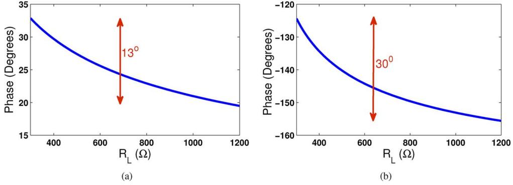
Fig. 9. Variation of phase of output with changing impedance settings for tapped capacitor match and  $\pi$ -match. (a) Tapped capacitor match. (b)  $\pi$ -match.
