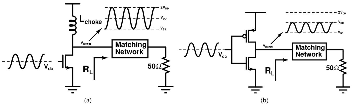
Fig. 7. Two canonical PA topologies considered. (a) NMOS-only PA topology. (b) Inverter-based push-pull PA topology.
