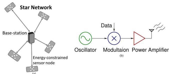
Fig. 1. (a) Star topology, a common network architecture for Body Area Networks. (b) The main blocks of a generic transmitter.
