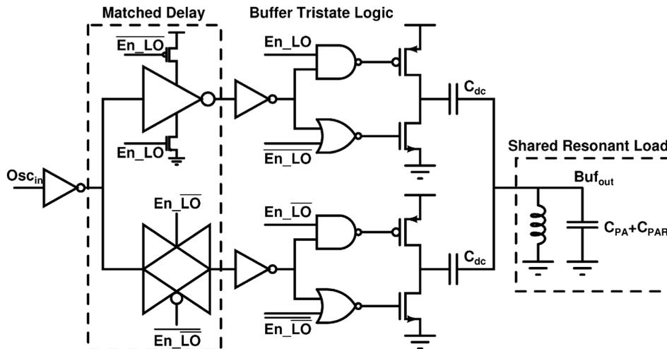
Fig. 6. Resonant Buffer with capability to generate  $LO$  and  $\overline{LO}$  for BPSK modulation.
