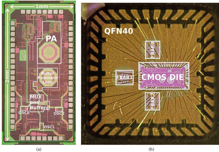
Fig. 12. Die photo of TX and the packaged chip with 3 FBARs. (a) Die photo. (b) Packaging photo.
