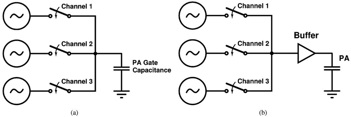
Fig. 4. Two multiplexing schemes. (a) Direct multiplexing of oscillators to PA. (b) Multiplexing of oscillators to PA with a buffer.
